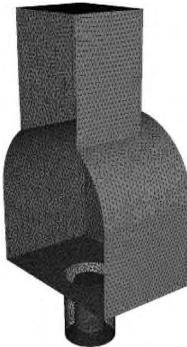
Fig. 2. Computational mesh: mesh generated by YAMS.
