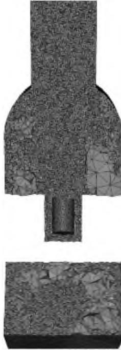
Fig. 5. Adapted meshes: cut through the tetrahedral mesh.
